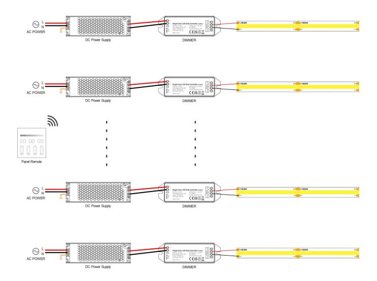
The dimmer can transmit the signals from the remote control to another dimmer within 30 meters. As long as there is a dimmer within 30 meters, the remote control distance can be limitless.
