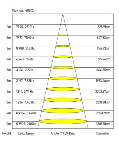
★ The curves indicate the illuminated area and the average illumination when the luminaire is at different distance.
