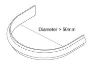
DO NOT bend LED strip to a diameter less than 50mm.
