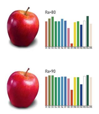
Ra evaluation index is applied to estimate the color rendering index of the lighting product to see the reflection level on natural color compared to those by conventional lighting.
