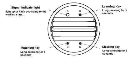
Code matching operation: the receiver will only be controlled by the value code remote control.
