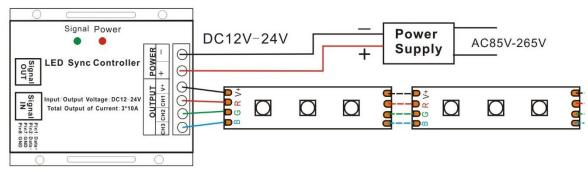
Application Circuit 2: (Synchronization function with network Line (RJ45))
