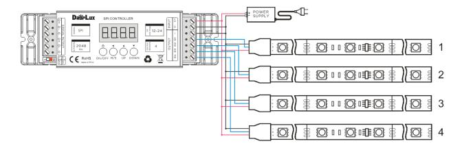
**Synchronization Circuit 2:** take the single-signal-wire digital led strip as an example
