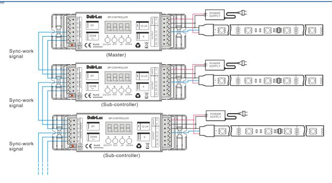
Note: The first one will be the master, please set the DIP switch to ON position; others from the second one will be the subcontrol, please keep the DIP switch in the factory default setting -OFF.
